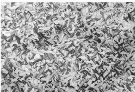
Figure 2. Optical textures under crossed polars of mesophases doped with (a) calcium acetate (b) phosphoric acid.
